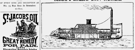
CTERNWHEEL STEAMERS have been found by experience to be the best type of vessel for shallow river navgration, of these Messes, Yarsow have constructed a faree number of successful examples for all parts of the world.
