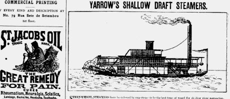
CTERNWHEEL STEAMERS have been found by experience to be the best type of vessel for shellow river navgation, and of these Messes. Yarnow have constructed a large number of successful examples for all parts of the world. Vessels on this system are constructed where required, to draw as little as 6 inches.
