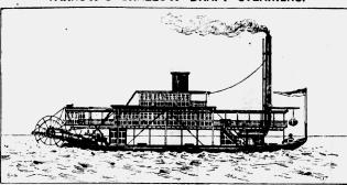
GTERNWHEEL STEAMERS have been found by experience to be the best type of vessel for shallow river navigation, and of these Messrs, Varkow have constructed a large number of sugcessful examples for all parts of the world. Vessels on this system are constructed when required, to draw a little as 6 inches.
