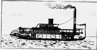
STERNWHEEL STEAMERS have been found by experience to be the best type of vessel for shallow river navigation and of these Mesers. Yannow have constructed a large number of successful examples for all parts of the world.
