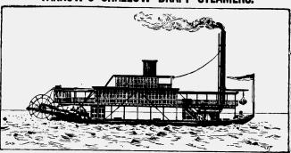
STERNWHEEL STEAMERS have been found by experience to be the best type of vessel for shallow river naviges and of these Messrs. Yaknow have constructed a large number of successful examples for all parts of the world. Vessels on this system are constructed when required, to draw as little as 6 many large for all parts of the world. Messrs. Yaknow lately built the sternwheelers "Mosquito" and "Herald" for the British Government, for see "the Yawnbea".
