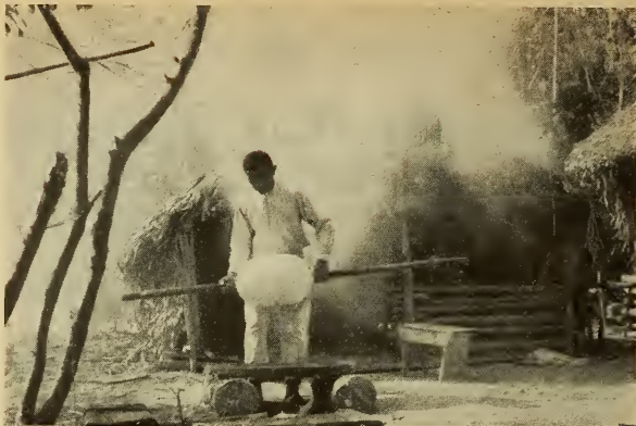
Curing rubber in the smoke of burning urucuri nuts
