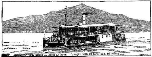
YARROW'S make a speciality of SHALLOW-DRAUGHT RIVER STEAMERS, either propelled by a STERN-WHEEL or by SCREWS WORKING IN TUNNELS, fitted with YARROW'S PATENT HINGED FLAP, by which means a considerable increase in speed is obtained without increase of cost. Vessels can be delivered whole, in pieces, or in floatable sections arranged so that they may be readily united while affoat.
