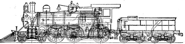
These locomotive engines are adapted to every variety of service, and are built accurately to mplates. Like parts of different engines of same class perfectly interchangeable. Passenger and arrow Gauge Locomotives, Steam Street Cars., &c., &c. (c. )
